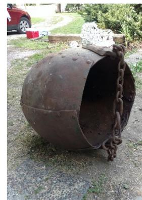
Kibble, barrel-shaped, ~ 3 ft. high and 2.5 ft. across top opening, an estimated weight of 250 lbs.
