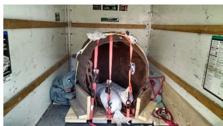
Kibble strapped to a wood base with sides wedged. Base strapped to corners and wedged against side of the trailer to avoid sliding. Weigh added to avoid tipping
