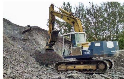
Excavator preparing a mine rock pile. Rock is moved and spread out with the goal to provide material not previously searched.
